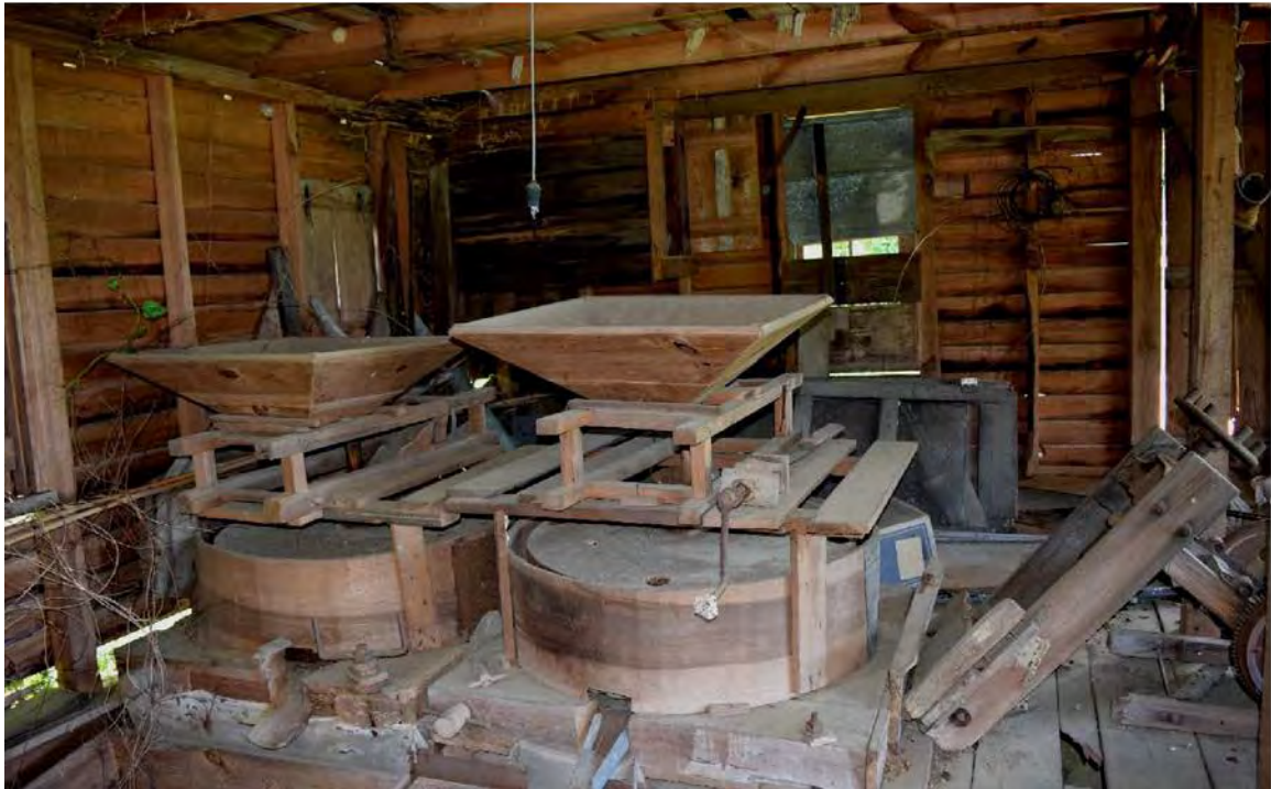
Figure 23. Millhouse addition southeast corner showing the two corn grinders on the entrance level wood floor.
